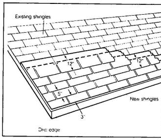
center of the strip. End nails should be 1-in. from the edges and both center nails should be 12-ins. in from the edges--as for field shingles.
