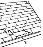
Use old shingles for alignment when installing a new asphalt strip roof over an old asphalt strip roof. Note in this example that the first course is only 3 ins. CAUTION: When working on a pitched roof, always wear rubber-soled shoes. It is
