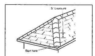
Hip shingles are laid in the same way as ridge shingles, but trim the end shingles at the eaves, edge, and ridge for the proper fit.
