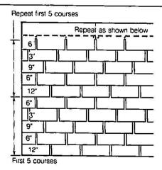
So-called random spacing is created by using this shingle pattern. The shingles must be cut in multiples of 3 ins. Start the first regular course of shingles with a full shingle.
